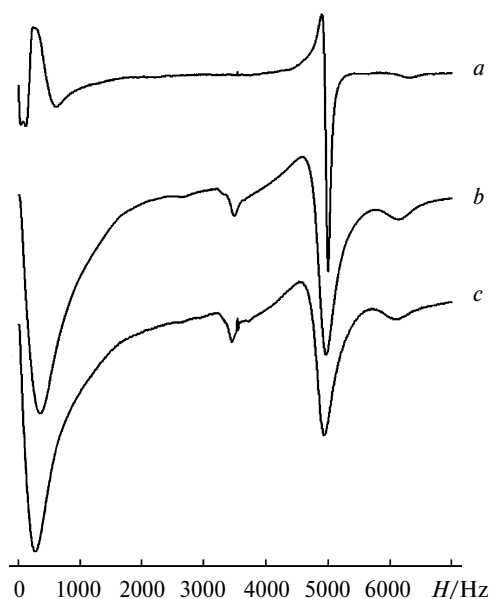
Fig. 3. X-band EPR spectra of polycrystalline samples of the copper complex [ \text{py}_2\text{Cu}_2(\text{piv})_4 ] ( a ) and compounds 1 ( b ) and 2 ( c ) at room temperature.
